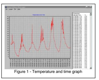
above the average. A max min thermometer would only show the peak without showing the average. The logger gives much more useful information than a simple thermometer.
