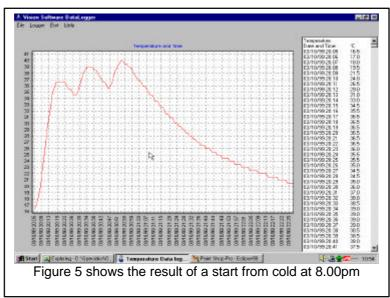
so that the warm air from the radiator metalwork would bathe the circuit with heat. Figure 5 shows the result of a start from cold at 8.00pm. The system warms up quite quickly, certainly more quickly that the fall in temperature as the boiler turned off at 9.00pm. Again the cycling of the boiler from on to off is clearly visible. The overall temperature rises over the hour; with the peaks continuing to rise.
