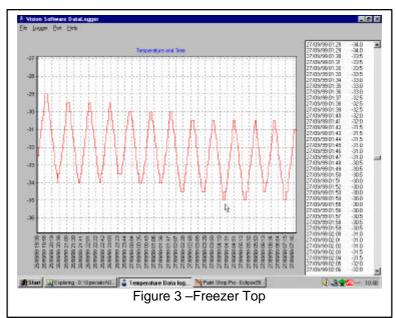
Figure 3 shows the plot of the top of the freezer. It shows a similar cycling effect to the fridge but the temperature difference is about 4°C compared with about 2°C for the fridge. The temperature is well below the -18°C target so the food should be OK. Figure 4 is a plot of the bottom of the freezer. It shows only a 0.5°C cycle so perhaps my cold air is showing its effect by falling to the bottom of the freezer! Any experts, could you please comment?
