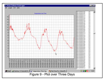
I chose a position, which was out of direct sunshine, on a concrete slab about 50mm above the level of the grass. Figure 9 shows the plot over three days or so. On each morning the temperature drops below 4°C but never gets to 0°C,
